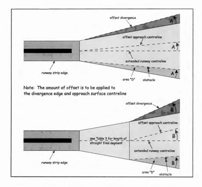
FIGURE 2 - OFFSET APPROACH SURFACE (NON-INSTRUMENT RUNWAYS)
